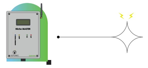
It is the brain of the whole system; the MASTER niche is used to collect information from the smart switch, gateway, energy meter and send it to the server and store it.
